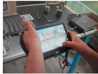
Fig. 24. A tablet used by the worker during the setup of a CNC grinding machine (source: [36,37,38]).
