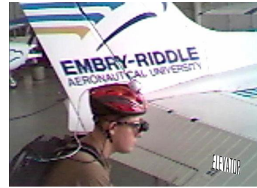
Fig. 3. A mobile AR system with HMD used in aircraft maintenance activities (source: [6]).
