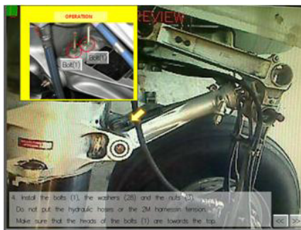
Fig. 6. Operator's view of the IAR system during the maintenance of an aircraft undercarriage (source: [10]).
