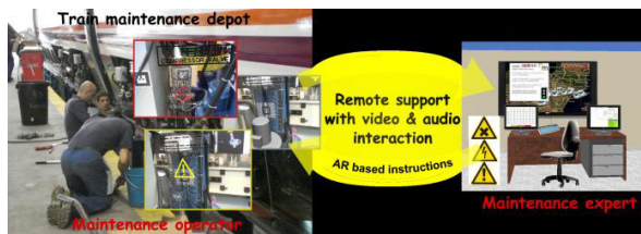
Fig. 15. Remote maintenance in a train depot using AR-based instructions (source: [24]).
