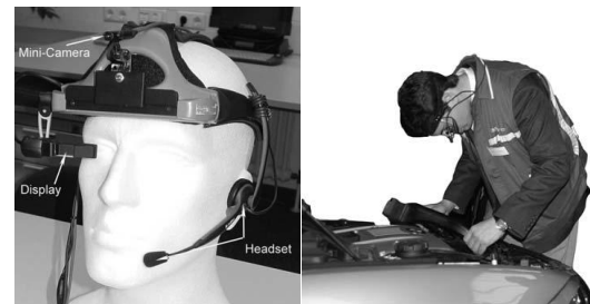
Fig. 7. Optical see-through HMD used in the maintenance procedure of a commercial vehicle (source: [12]).
